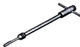
Choose the tool No.9, there are a hex 12 mm bolt and 30 mm hex nut and a cone center tool. Screw the No.12 bolt (1/4"-28 UNF Hex 9 mm) into the hex 12 mm spindle and use a 9 mm spanner to tighten the No.12 bolt. Install the cone center tool & hex 12 mm bolt into glow plug hole; then screw the M30 hex nut properly. Use M12 spanner to fix the hex 12 bolt head and use the M30 spanner to turn the M30 hex nut clockwise to extract the rest part of glow plug:
