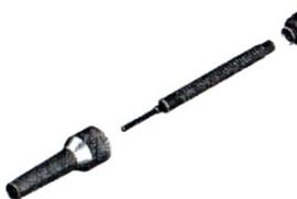
Choose a tap (M10 x P1.0 or M8 x 1.0) from No.8, install it with T-handle, and tap the glow plug hole.
