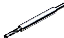
Separate the No.9 device and only choose the cone center tool and install it into the glow plug hole. Choose suitable drill from No.2/3 (7 x 5.5 or 9 x 5.5), insert the drill into No.13 (drill installer). It is important to use No.11 (3 mm alley key) to lock the screw on drill installer. Then install it into cone center tool and connect with air tool to drill and also remove the hex nut from glow plug.
