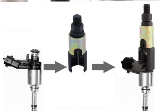
The new nozzle(s) and all dismantled components can then be reassembled. In addition, the fuel filter should also be changed directly to prevent soiling in the system.
