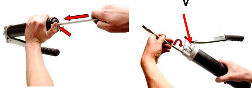
Press the Valve (V) and press pump lever several times, to push air out of the grease gun.
