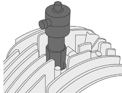
3. Loosen fixing screw.
