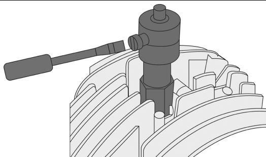
6. Turn the crankshaft a half a rotation against the "normal" direction of rotation.
